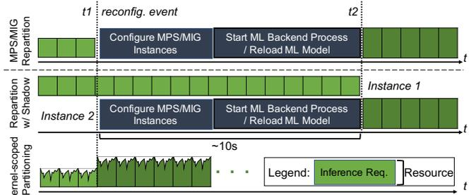
Fig. 2: Resizing inference server’s spatial partition. Existing commercial GPU spatial partitioning techniques are enforced at the process-level. (Top) Reconfiguring spatial partition size requires restarting the ML backend and reloading models. (Center) Prior works mask this downtime by reconfiguring shadow instances, but repartitioning is still limited to every ~10s. (Bottom) Our work enables inference requests and kernels within requests to instantaneously resize spatial partitions.
