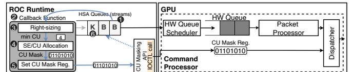
(b) Emulation implementation details built on AMD’s CU Masking.
