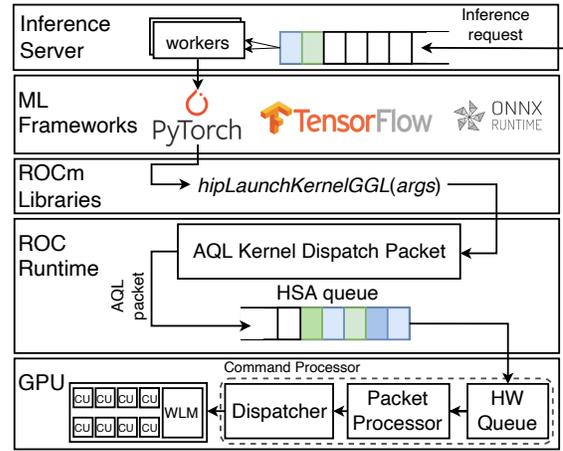
Fig. 9: Overview of an AMD GPU-based inference server.
